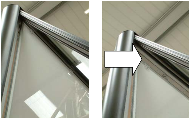
Fig. 3.2.1. Diffuser drop down
